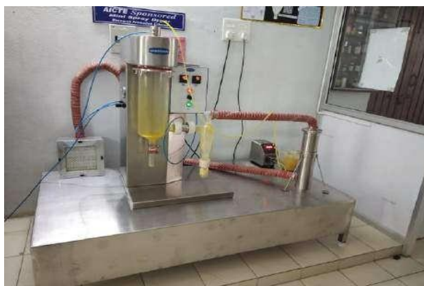
Fig.12 spray drying of herbal extracts
