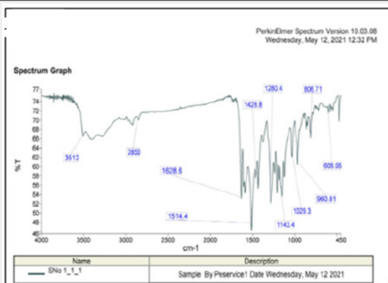
Figure 15: FTIR spectra of pure curcumin.
