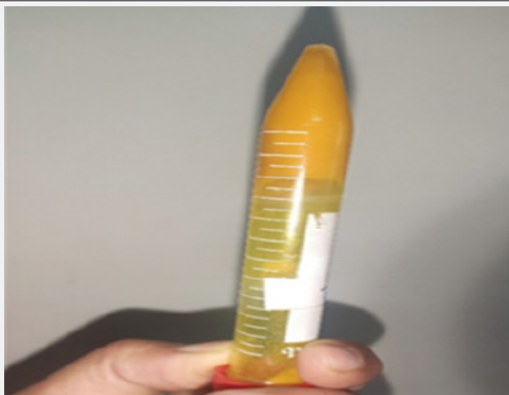
Figure 6: Image of in-situ gelling system when kept at room temperature for some time.
